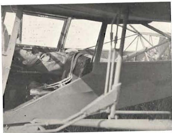
Ambulance work. The stretcher is loaded into the cabin on a special guide ramp.
