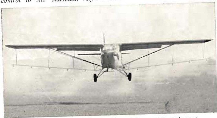
An Auster "Aiglet" fitted with aerial spraying equipment.
